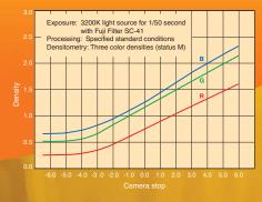
In order to simulate conditions closest to practical use, exposure was made under a 3200K tungsten light source, through a Fuji SC-41 ultraviolet absorbing filter. Processing was carried out under standard conditions and the three color densities were measured, producing the results indicated in the graph above.
