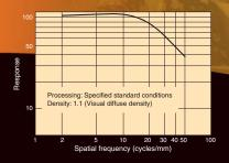
\* Spatial frequency attenuation characteristic of amplitude relative to rectangular wave chart. (Data is normalized for amplitude of zero frequency.)
